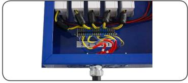
Refer to wiring diagram at the back of the cover of the ballast box. Using a small screw driver, press in the latch and insert the appropriate wire in the terminal block connector then release the screw driver. The wires should hold firmly into the terminal block connector.
