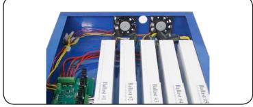
Each set of 4 wires (2 blue and 2 yellow) are labelled 1 to 5 and correspond to lamp 1 to lamp 5. Ballasts 1 to 5 are labelled accordingly and lamps 1 to 5 are identified on the terminal block where the associated wires should connect.
